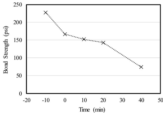
**Figure 4. Bond strength vs. placement delay**
