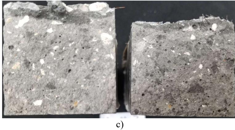
Figure 5: Failure Types: a) SCC Failure, b) UHPC Failure and c) Interface Failure
