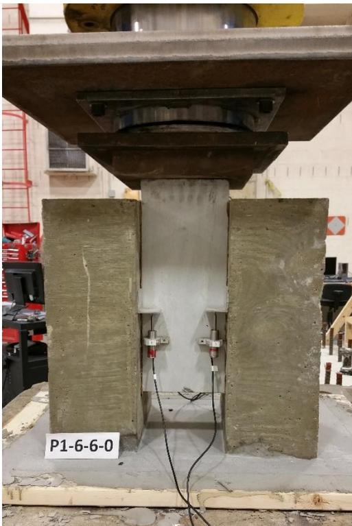
**Figure 2. Large-scale, double shear push-off specimen**
