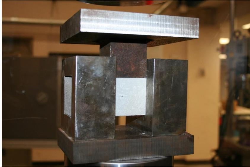
**Figure 1. Small-scale, beam-like double shear specimen**
