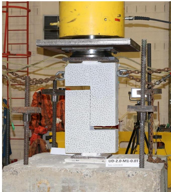
**Figure 3. Large-scale, single shear push-off specimen**
