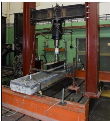
Figure 6. View of the testing frame for bend test
