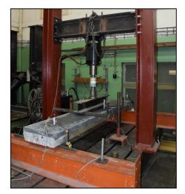
Figure 6. View of the testing frame for bend test
