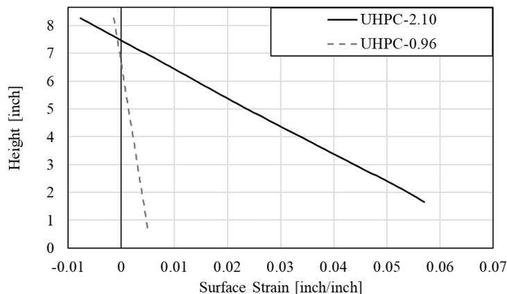
**Figure 7. Measured Surface Strain Along the Beam Height at Peak Load**
