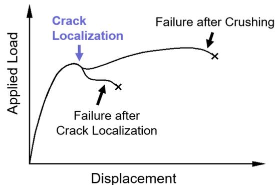
Figure 1. Schematic of the Two Failure Paths
