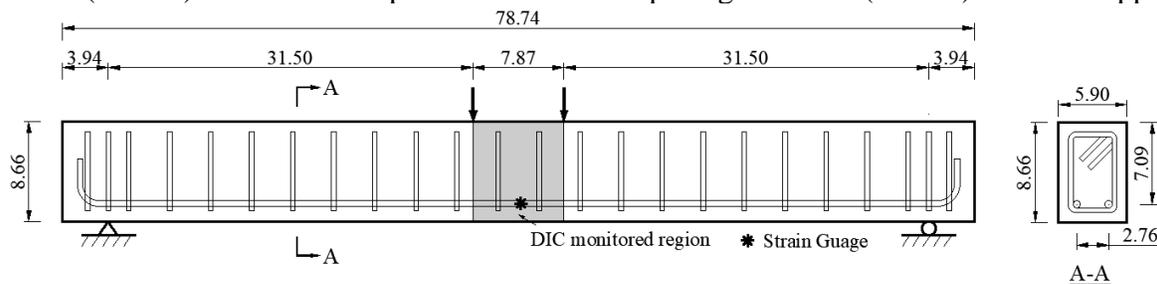
**Figure 3. Specimen Design and Test Setup. (Unit: inch; 1 inch=25.4 mm)**
