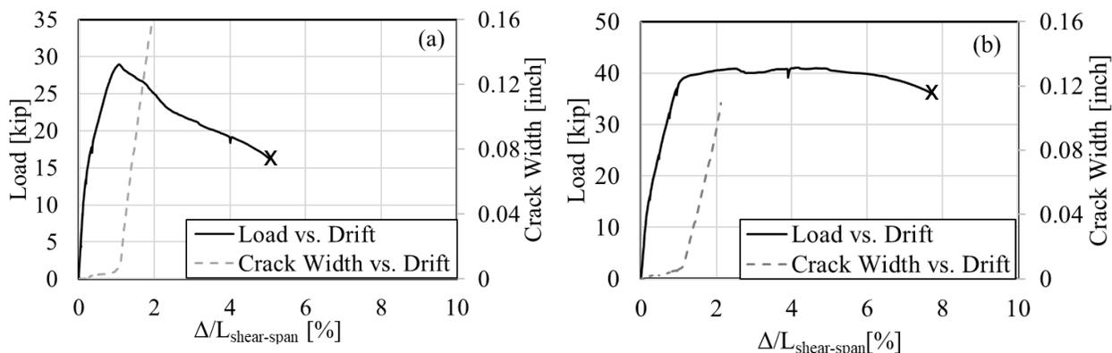
**Figure 4. Load-drift Response and Maximum Crack Width History for: (a) Beam UHPC-0.96, and (b) Beam UHPC-2.10. (1kip=4.44 kN; 1 inch=25.4 mm; 'X' represents reinforcement fracture)**
