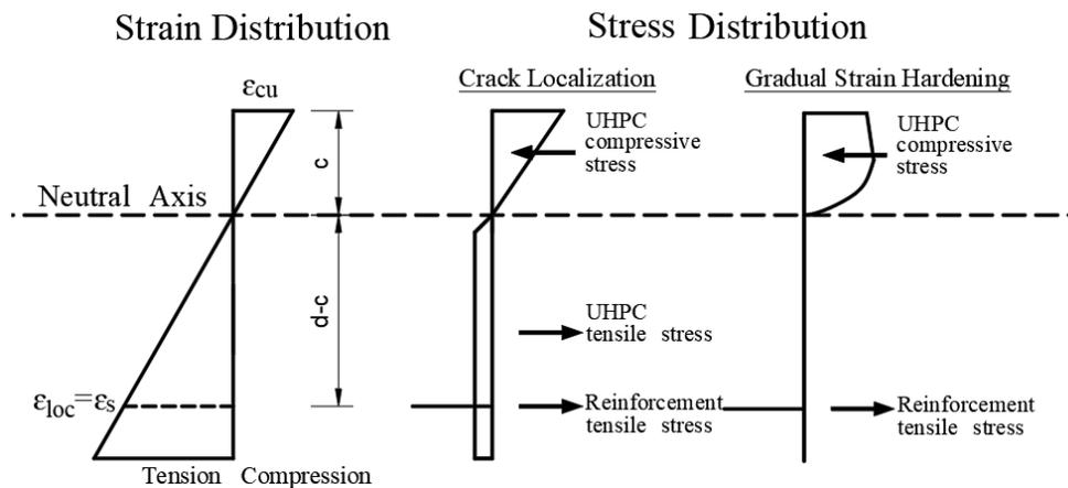
**Figure 8. Strain and Stress Distributions for a Proposed Flexural Strength Prediction Method.**
