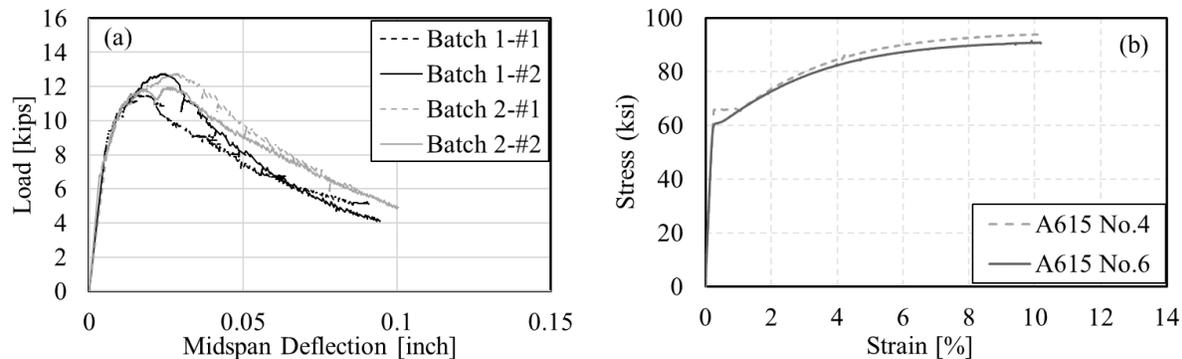
**Figure 2. Material Behavior: (a) Load-deflection Response of the Unreinforced UHPC Beams; (b) Tensile Stress-strain Response for the Longitudinal Reinforcing Steel. (1kip=4.44 kN, 1 inch =25.4 mm)**
