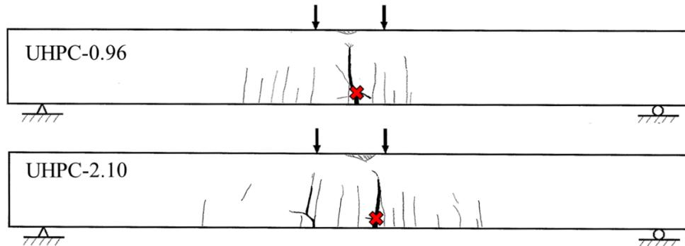
Figure 5. Crack Pattern before Reinforcement Fracture ('X').
