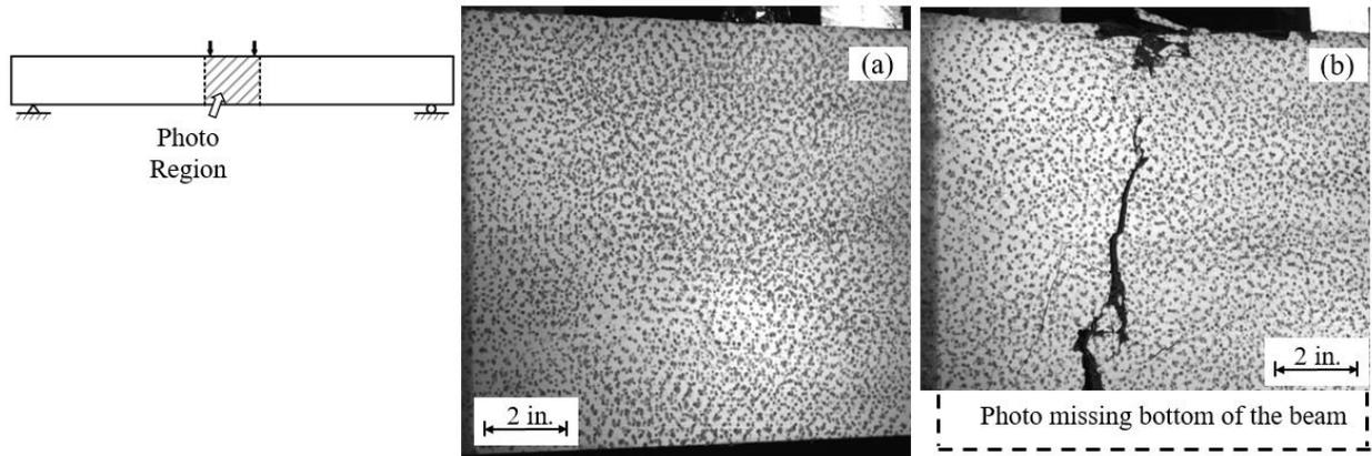
**Figure 6. Cracking Behavior of Constant Moment Region at Peak Load for beams (a) UHPC-0.96, and (b) UHPC-2.10. (1 inch=25.4 mm)**
