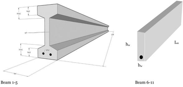
Figure 1. Geometrical parameters of beams
