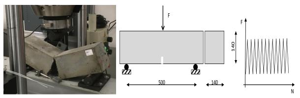
Figure 7. Fatigue test under UHPC
