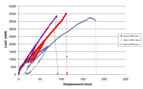
Figure 4. Load -displacement curve Beam 1 to 3
