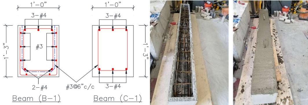
Figure 1: Reinforcement detail and construction of specimen
