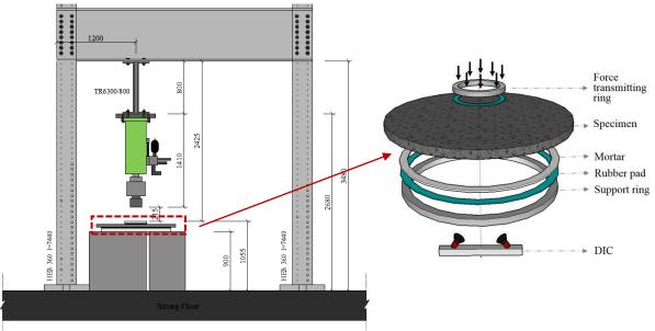
Figure 1. Schematic description of test setup
