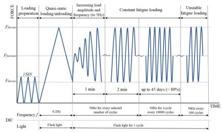
Figure 2. Qualitative fatigue loading history and DIC measurement program
