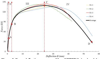
Figure 3. Force-deflection response of four UHPFRC circular slabs
