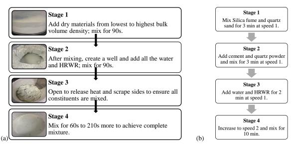
Figure 2 The 4-stage mixing protocols for a) the resonance acoustic mixer and b) the table top paddle mixer.
