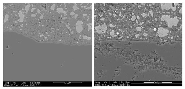
Figure 4 The interfacial transition zone for a Hobart (left) and a RAM (right) specimen.
