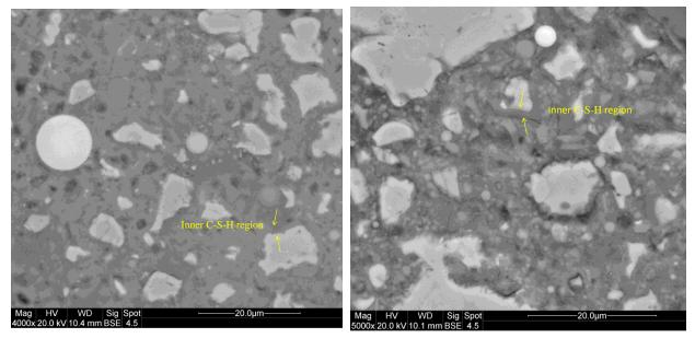
Figure 3 Inner C-S-H region is lighter around the Hobart (left) than the RAM (right) for the samples.
