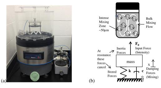
Figure 1 (a) The acoustic laboratory size mixer LabRAM and (b) the schematic of its mixing technology (S L Coguill).
