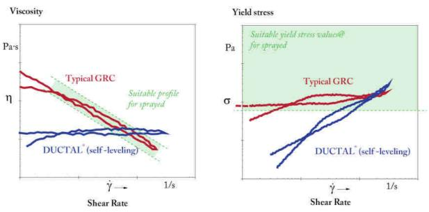
Figure 4. Fresh state comparison between a self-compacting Ductal<sup>®</sup> and typical GRC
