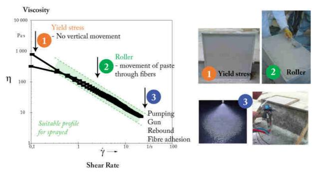
Figure 3. Schematic description of expected fresh state behavior for the GRC process
