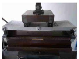
Figure 7. Four bending test on a sprayed Ductal<sup>®</sup> thin plate
