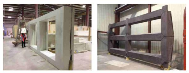
Figure 6. Example of 3D panel produced by Betsinor (France)
