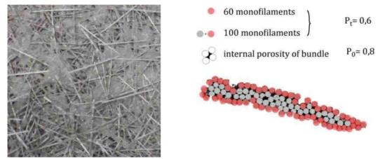
Figure 8. Random orientation of glass fibers after spray
