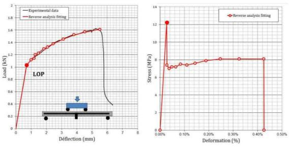
Figure 10. Flexural loading versus deflection curve and Uniaxial tensile stress versus strain curve after back analysis
