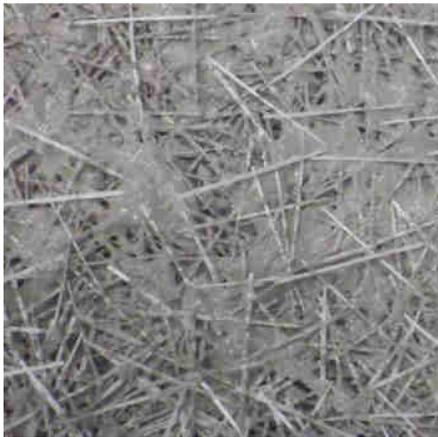
Figure 8. Random orientation of glass fibers after spray
