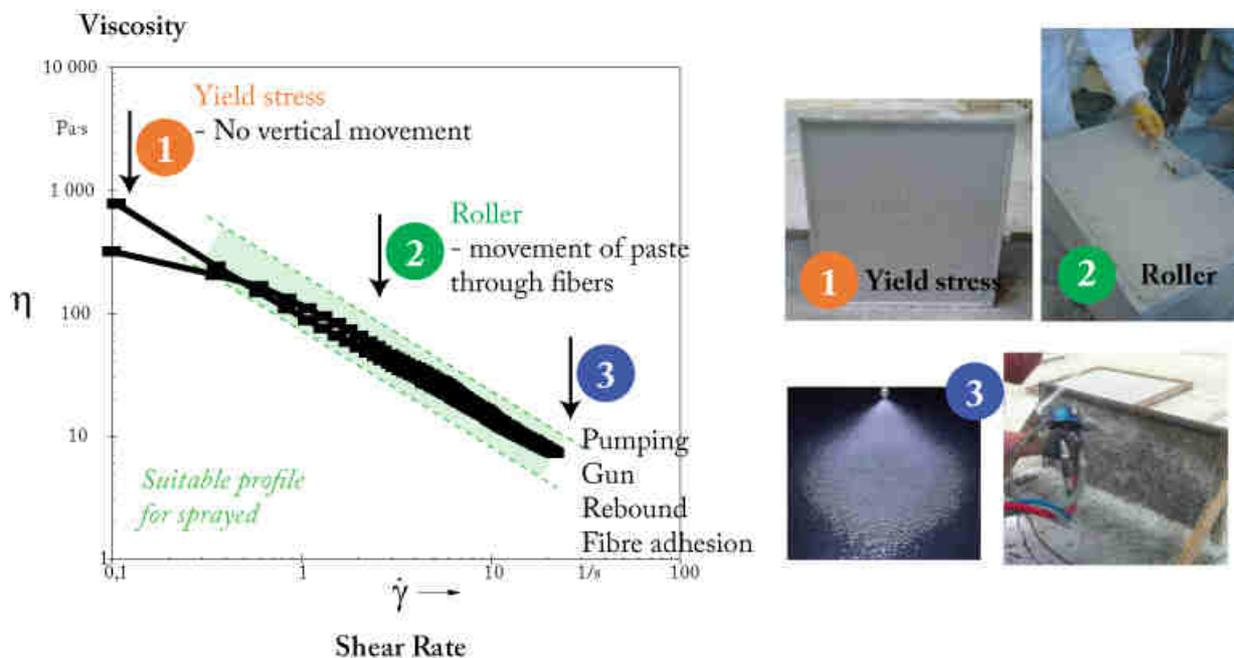
Figure 3. Schematic description of expected fresh state behavior for the GRC process
