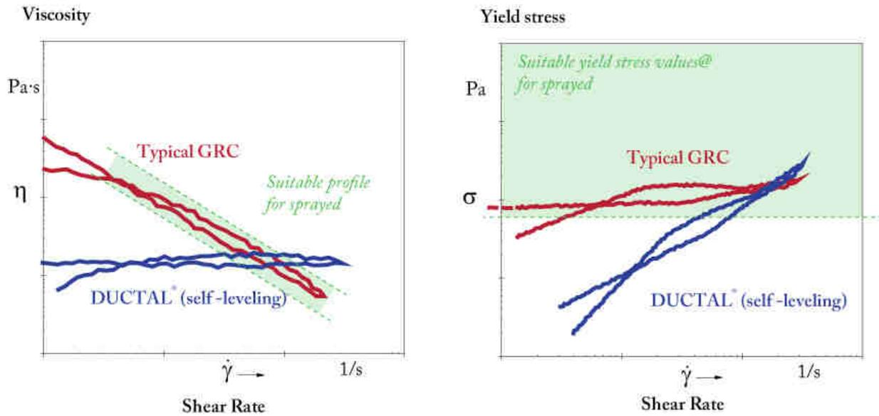
**Figure 4. Fresh state comparison between a self-compacting Ductal® and typical GRC**
