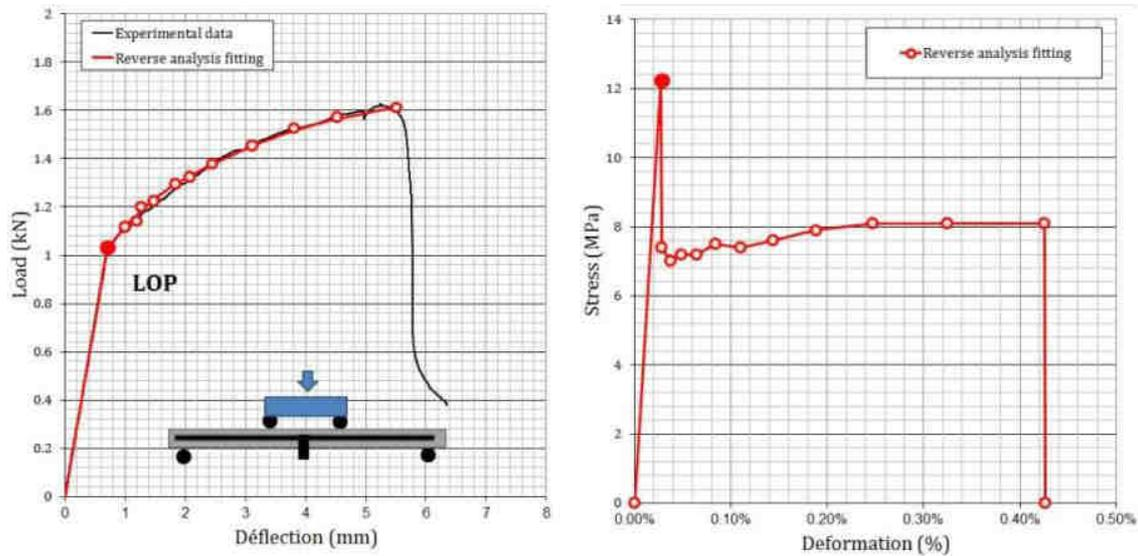
**Figure 10. Flexural loading versus deflection curve and Uniaxial tensile stress versus strain curve after back analysis**
