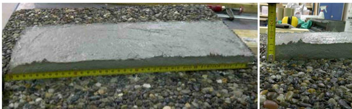
**Figure 8. Fresh Ductal® poured on a 7% sloped rough plate (dimensional control)**
