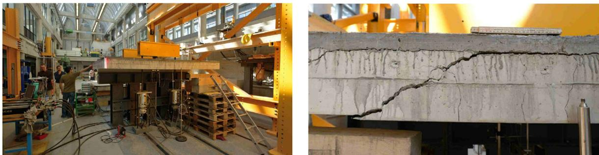
**Figure 4. Bending and shear tests on composite slabs reinforced with strain-hardening UHPFRC**
