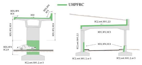
Figure 3. Concepts of application of the local strengthening of structures with UHPFRC
