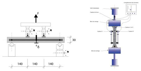
Figure 7. Bending and direct tensile tests on strain-hardening Ductal<sup>®</sup> specimens
