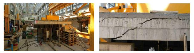
Figure 4. Bending and shear tests on composite slabs reinforced with strain-hardening UHPFRC
