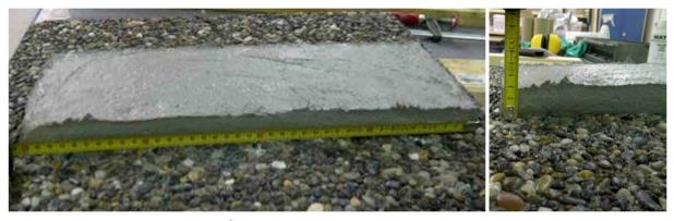
Figure 8. Fresh Ductal<sup>®</sup> poured on a 7% sloped rough plate (dimensional control)
