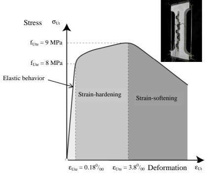
Figure 9. Direct tensile behavior of strain-hardening Ductal®
