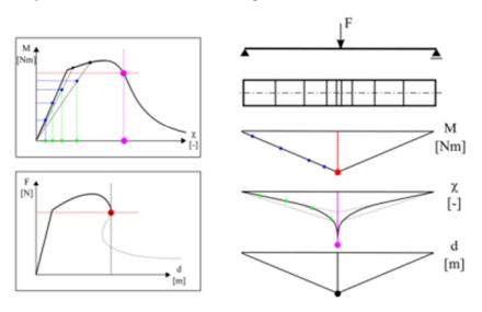
Figure 10. Principles of the curvature-based formulation
