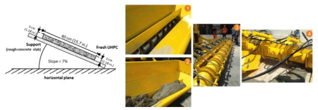
Figure 6. Slope test and scale-up test with the casting machine
