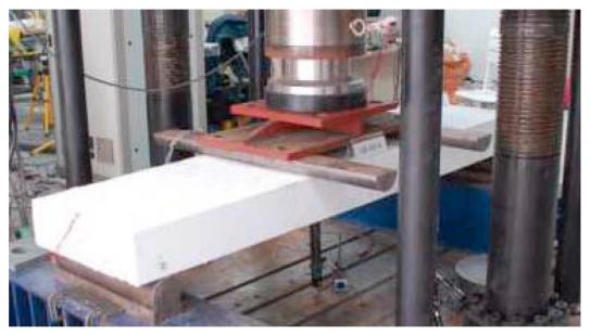
Figure 2. 4-Points bending test
