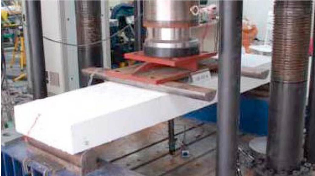
Figure 2. 4-Points bending test
