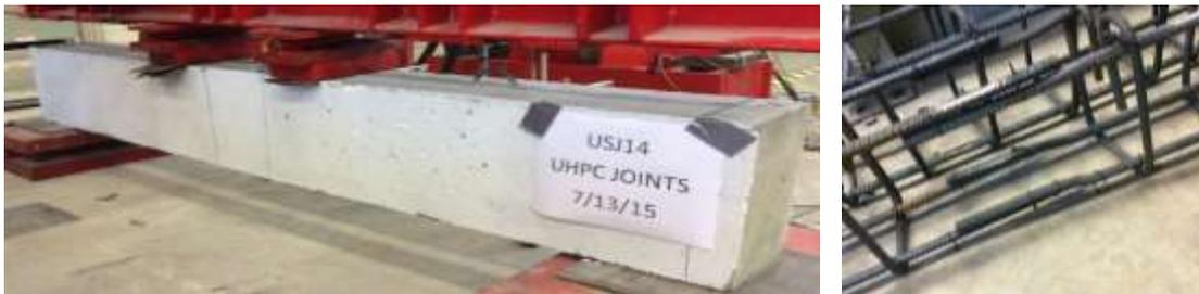
**Figures 1 & 2. Specimen during testing, straight-lap reinforcement detail in the joint**
