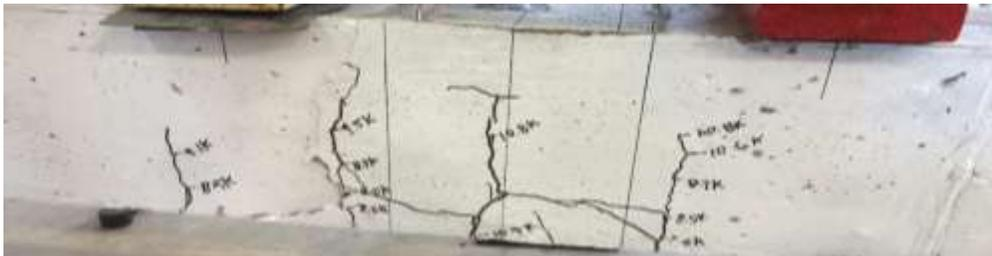
**Figure 10: HS-SCC joint beam after failure**
