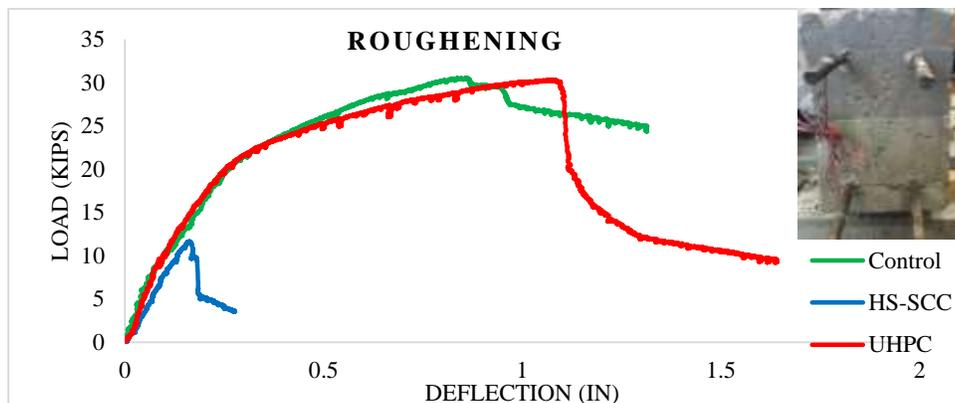
Figure 7: Load versus deflection plot for Rough surface preparation
