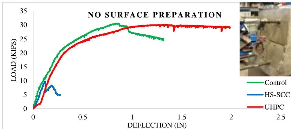
Figure 6: Load versus deflection plot for No surface preparation
