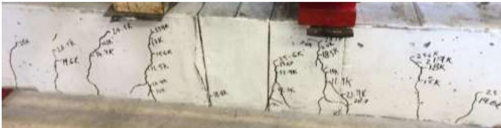
**Figure 11: UHPC joint beam after failure**
