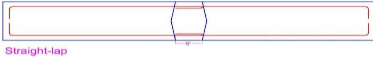
Figure 4. Reinforcement detail of joint for all specimens
