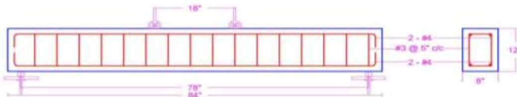
**Figure 3. Reinforcement Detail of Control**
