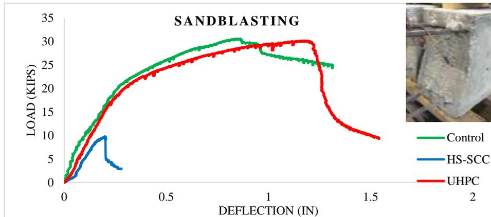
**Figure 8: Load versus deflection plot for Sand blasted surface preparation**
