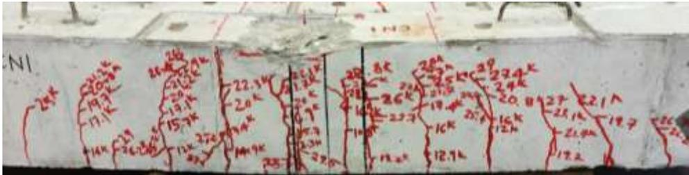
**Figure 9: Control beam after failure**
