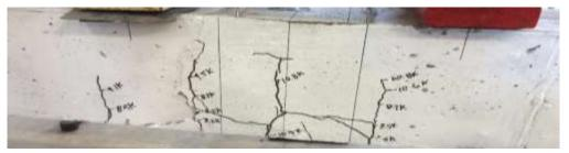
Figure 10: HS-SCC joint beam after failure
