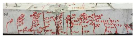
Figure 9: Control beam after failure
