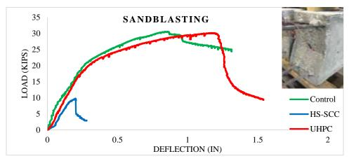
Figure 8: Load versus deflection plot for Sand blasted surface preparation
