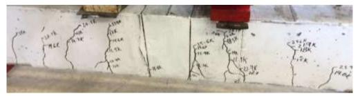
Figure 11: UHPC joint beam after failure
