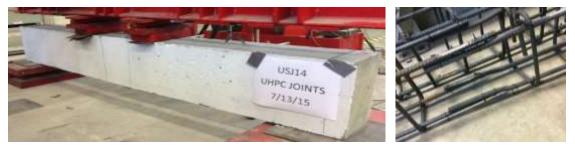
Figures 1 & 2. Specimen during testing, straight-lap reinforcement detail in the joint
