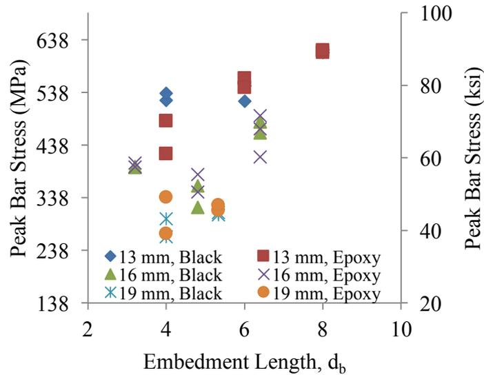
**Figure 3: (a) Peak Bond Stress Achieved vs. Embedded Length and (b) Peak Bar Stress vs. Embedded Length, 2% fiber vol., Parallel Fiber Orientation, 28 days cured**
