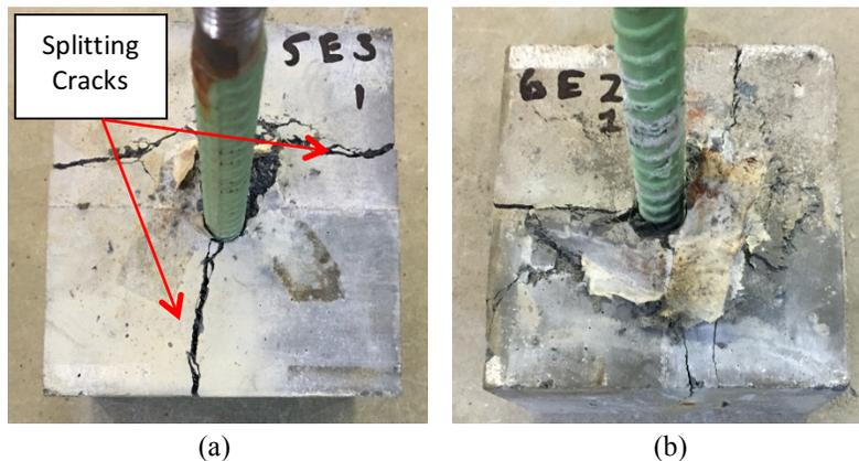
**Figure 1: (a) Bar Slip, and (b) Conical Concrete Failure**
