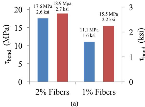
**Figure 4: (a) Peak Bond Stress Achieved at 1% and 2% Fibers by volume: 19 mm bars, Embedded 4.0  $d_b$  (Blue) and 16 mm bars (Red), Embedded 6.0  $d_b$**
