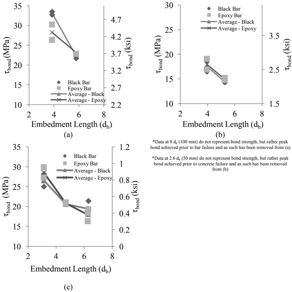
**Figure 2: (a) Peak Bond Stress vs. Embedment Length in  $d_b$  for 13 mm bars, (b) 16 mm bars and (c) 19 mm bars**
