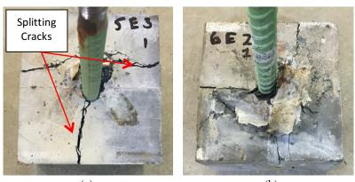
(a) (b) Figure 1: (a) Bar Slip, and (b) Conical Concrete Failure
