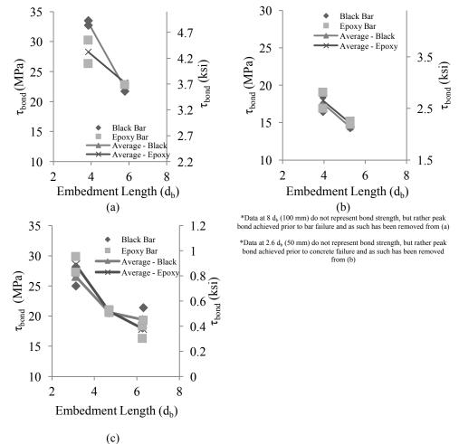
Figure 2: (a) Peak Bond Stress vs. Embedment Length in d<sub>b</sub> for 13 mm bars, (b) 16 mm bars and (c) 19 mm bars
