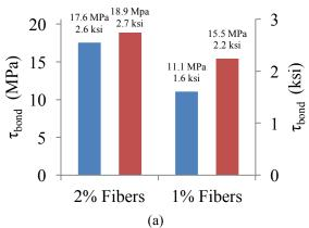
Figure 4: (a) Peak Bond Stress Achieved at 1% and 2% Fibers by volume: 19 mm bars, Embedded 4.0 d<sub>b</sub> (Blue) and 16 mm bars (Red), Embedded 6.0 d<sub>b</sub>
