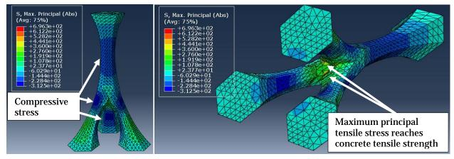
Figure 5. Finite element model and analysis result of three-legged columns
