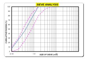
Figure 1. Grading curve of natural river sand
