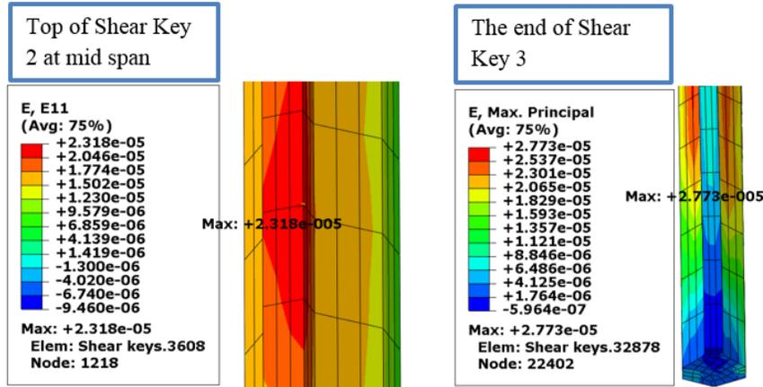
**Figure 7. Transverse Strain and Maximum Principal Tensile Strain for Load Configuration 4**
