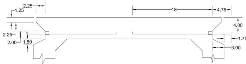
**Figure 2. Longitudinal Connection's Details, (all dimensions in inches, 1 in. = 25.4 mm)**
