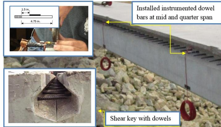
**Figure 4. Instrumenting and Installed a Shear Key Dowel Bar and Shear Key with Dowels (all dimensions in inches, 1 in. = 25.4 mm)**
