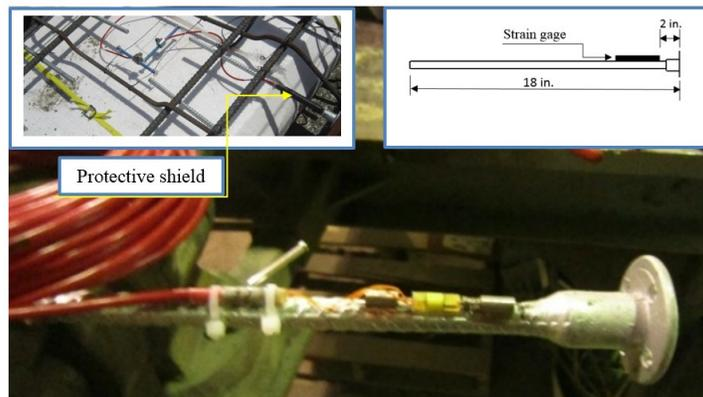
**Figure 3. Instrumented Dowel Bar and Dowel Bar Covered with a Protective Shield, (all dimensions in inches, 1 in. = 25.4 mm)**
