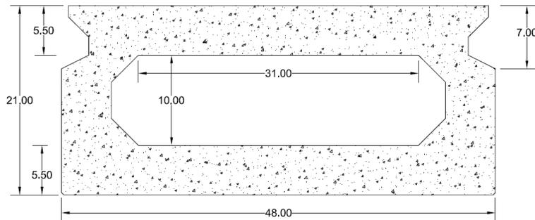
**Figure 1. Cross Section's Details, (all dimensions in inches, 1 in. = 25.4 mm)**
