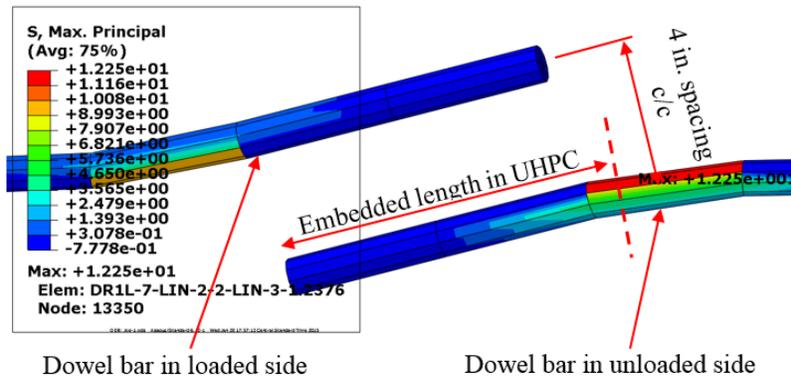
**Figure 8. Maximum Principle Tensile Stresses in the Dowel Bars for Load Configuration 4, (1 ksi= 6.895 MPa & 1 in.=25.4 mm)**
