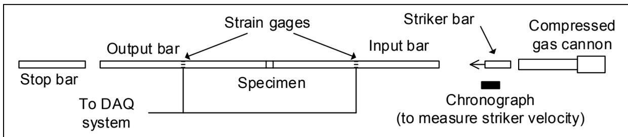
Figure 1. Diagram of the SHPB setup
