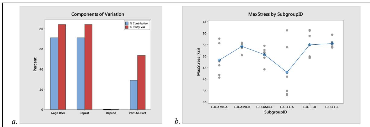
Figure 2. *a.* Gage R&R results for Cor-Tuf. *b.* Plot of maximum stress by group. Note: 1 ksi = 6.895 MPa
