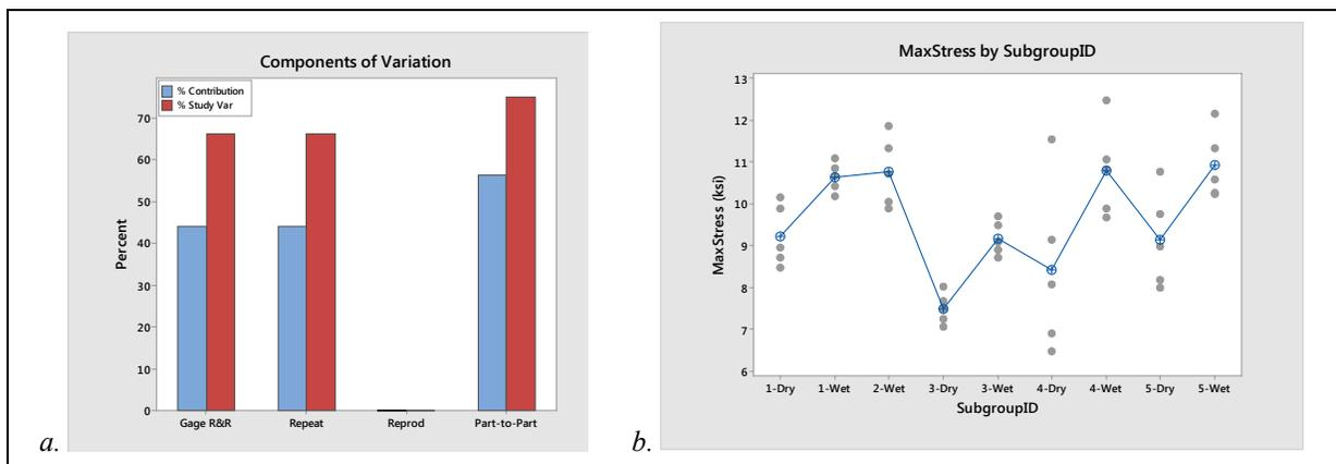
Figure 4. a. Gage R&R results for NSC. b. Plot of maximum stress by group. Note: 1 ksi = 6.895 MPa
