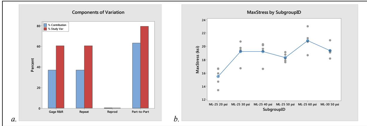
Figure 5. a. Gage R&R results for maple. b. Plot of maximum stress by group. Note: 1 ksi = 6.895 MPa
