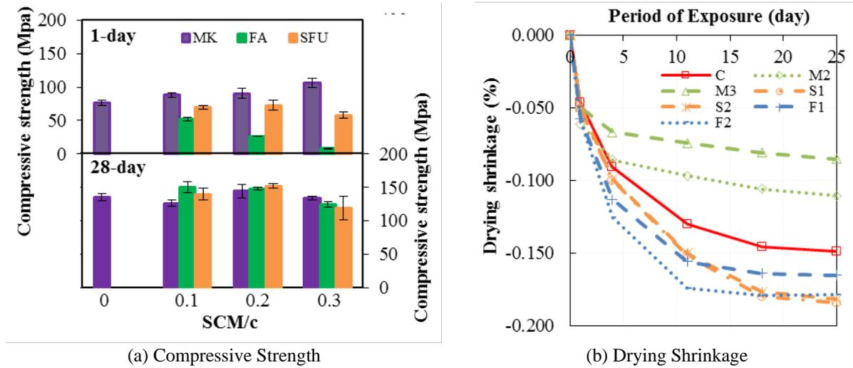
**Figure 3. Hardened State Properties of Paste Using Binary Blend of SCM and Cement**
