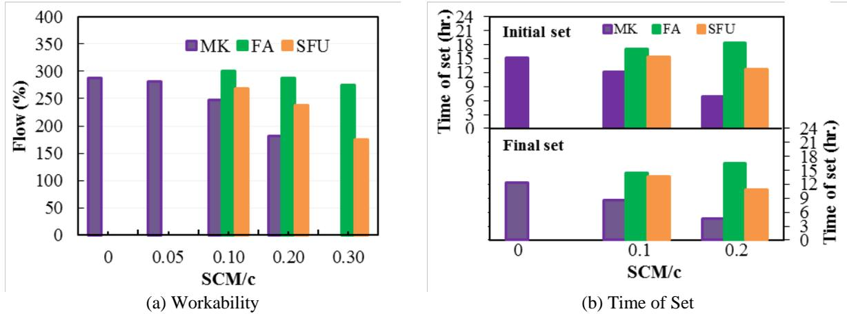
**Figure 1. Fresh State Properties of Paste Using Binary Blend of SCM and Cement**
