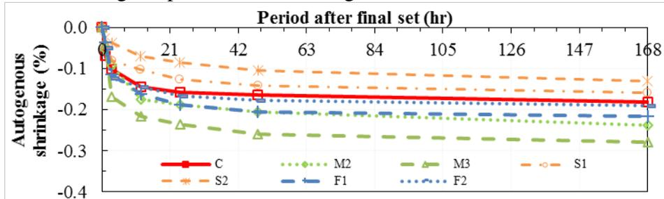
**Figure 2. Autogenous Shrinkage of Paste Using Binary Blend of SCM and Cement**
