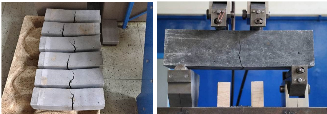
Figure 2. Specimens after the failure / experimental setup
