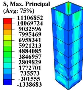
Figure 5. Distribution of maximum principle stress.
