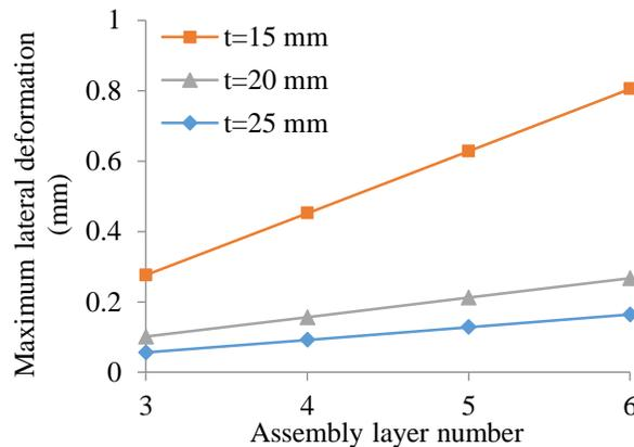
**Figure 8. Effects of assembly layer number and wall thickness on lateral deformation.**
