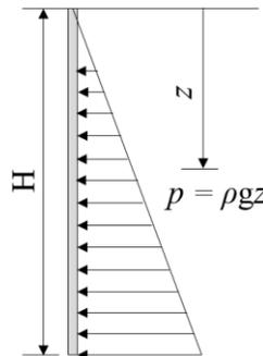
Figure 2. Illustration of static hydraulic pressure applied on SIP formwork.
