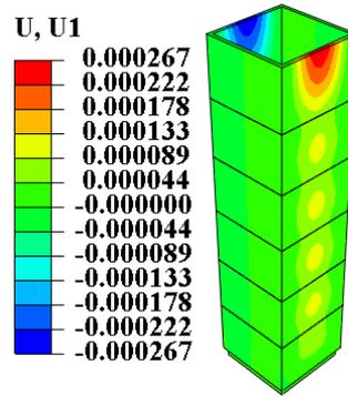
**Figure 7. Distribution of lateral deformation.**
