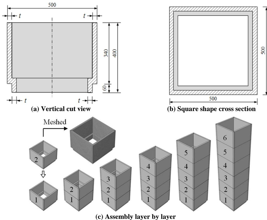
Figure 1. Illustration of the SIP formwork system.
