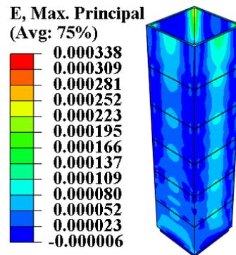
**Figure 3. Distribution of maximum principle strain.**
