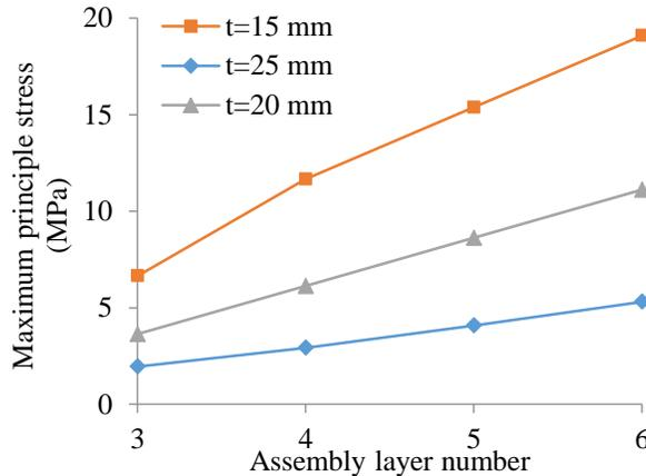
Figure 6. Effects of assembly layer number and wall thickness on maximum principle stress.
