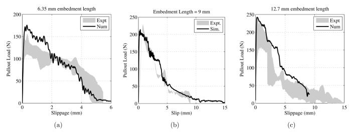
Figure 6. Effects of embedment length: (a) 6.35 mm embedment length, (b) 9 mm embedment length, and (c) 12.7 mm embedment length.
