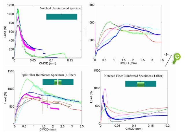
Figure 4. Test results for load vs. CMOD curves for three different configurations for the 4fiber case.
