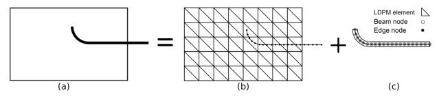
Figure 5. Kinematic model of fiber pullout test. (a) concrete specimen and fiber; (b) masterslave constraint between matrix (LDPM mesh) and fiber tunnel (geometric edge list); (c) penalty constraint between tunnel edge list and fiber (beam list).
