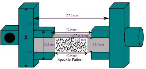
*Figure 2. Dimensions of the specimen.* Computer-Controlled MTS Testing Digital Image Correlation
