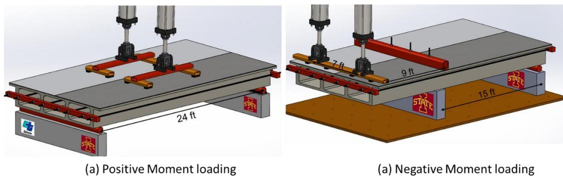
Fig. 2 The test setup planned for fatigue load evaluation.
