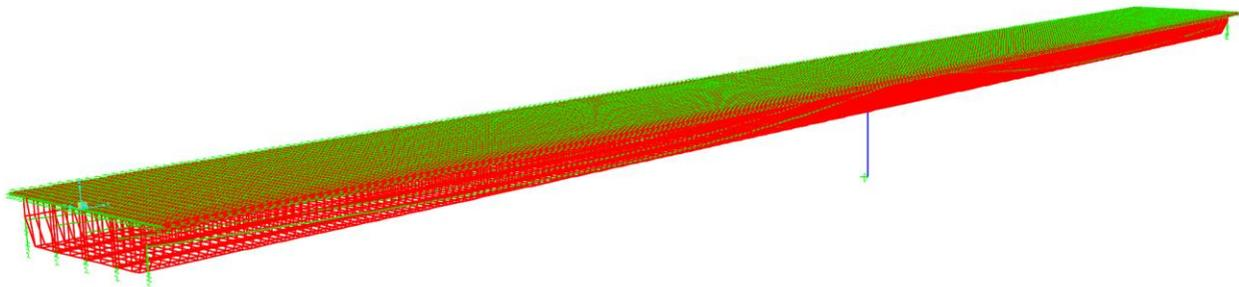
Fig. 1 Model of a two-span PTBG bridge with a thin layer of UHPC added to the deck.
