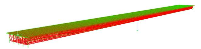
Fig. 1 Model of a two-span PTBG bridge with a thin layer of UHPC added to the deck.
