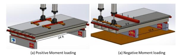
Fig. 2 The test setup planned for fatigue load evaluation.
