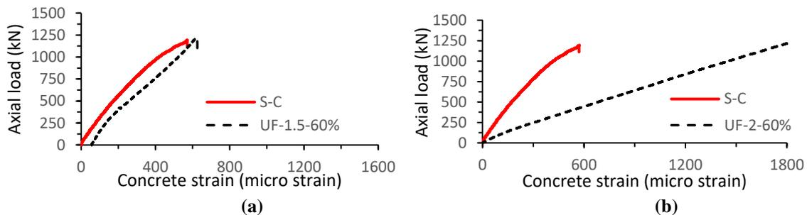
Figure 5: Axial load versus jacket concrete hoop strain of piers with jacket thickness of (a) 31 mm (1.5 inches) and (b) 51 mm (2 inches) (1 kN = 224.8lb)
