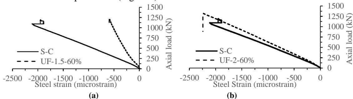
Figure 4: Steel strain of piers-jacket thickness (a) 38 mm (1.5 inch) and (b) 51 mm (2 inch) (1 kN = 224.8lb)
