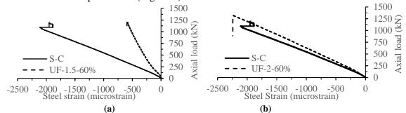
Figure 4: Steel strain of piers-jacket thickness (a) 38 mm (1.5 inch) and (b) 51 mm (2 inch) (1 kN = 224.8lb)
