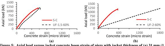
Figure 5: Axial load versus jacket concrete hoop strain of piers with jacket thickness of (a) 31 mm (1.5 inches) and (b) 51 mm (2 inches) (1 kN = 224.8lb)
