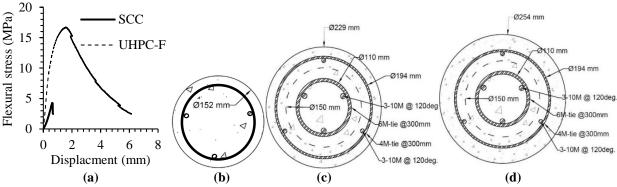
Figure 1: (a) Stress-deflection responses of SCC/UHPC and dimensions and reinforcement details of piers (b) core, (c) with 38 mm (1.5 inch), (d) 51 mm (2 inch) jacket layer (1 inch = 25.4 mm; 1 MPa = 145 psi)
