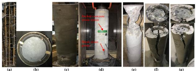
Figure 2: (a) Jacket reinforcements, (b) damaged SCC core pier in tube form, (c) repaired piers, (d) test setup with instrumented and failure pattern of piers (e) core (S-C), (f) jacketed UF -1.5-60%, (g) UF-2-60%
