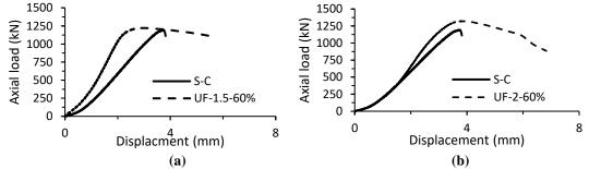
Figure 3: Load-displacement responses of piers -jacket thickness (a) 1.5 inch (38mm) and (b) 2 inch (51 mm)
