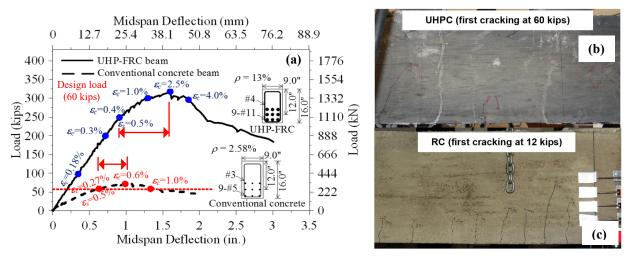
Figure 7: (a) load versus mid-span deflection responses of RC and UHPC beams, (b) observed cracks in UHPC beam at 300-kip (1334 kN) load, and(c) observed cracks in RC beam at 70-kip (311 kN) load
