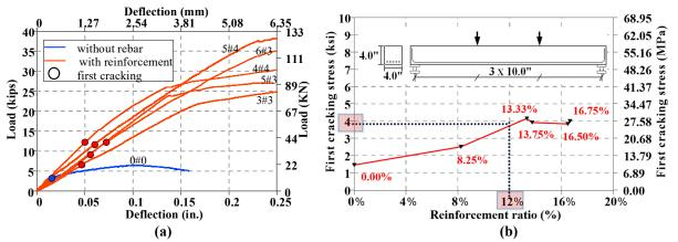
Figure 6: (a) test results, (b) first cracking stress versus reinforcement ration ( $\rho_{TA}$  = rebar area divided by the "tributary area of concrete" = 2 × cover thickness × width of beam)
