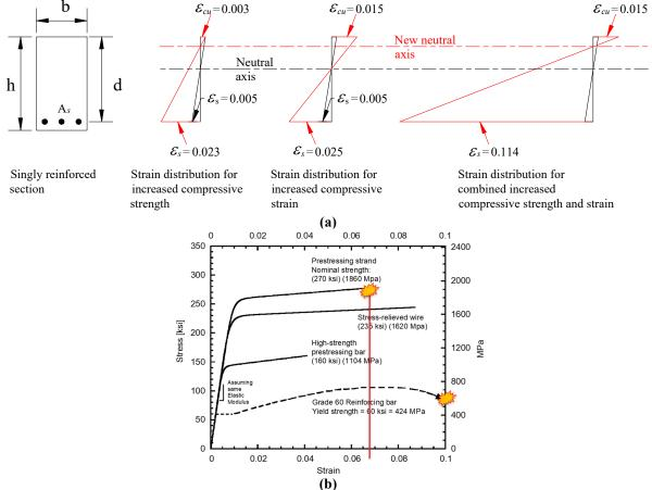
Figure 5: (a) tensile strain demands in the longitudinal steel reinforcement caused by the maximum compressive strain of UHPC, (b) strain capacities of typical prestressing strands and rebars
