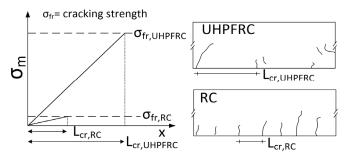
Figure 8: Crack spacing in RC beam and UHPC beam designed with high steel ratio
