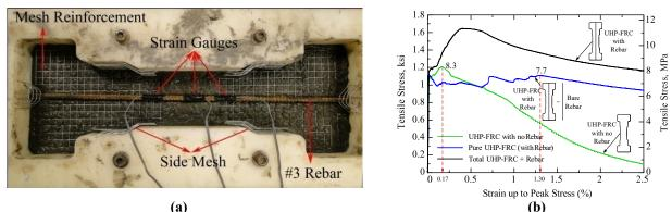
Figure 3: (a) the tensile specimen with one #3 rebar, (b) tensile stress-strain curves
