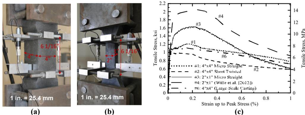
Figure 1: (a) large-scale tensile specimen (16.0 in.<sup>2</sup> [10,323 mm<sup>2</sup>]), (b) small-scale tensile specimen (2.0 in.<sup>2</sup> [1,290 mm<sup>2</sup>]), and (c) tensile stress-strain curves of UHPCs with different specimen sizes
