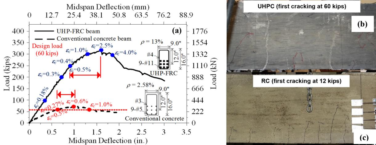
Figure 7: (a) load versus mid-span deflection responses of RC and UHPC beams, (b) observed cracks in UHPC beam at 300-kip (1334 kN) load, and (c) observed cracks in RC beam at 70-kip (311 kN) load
