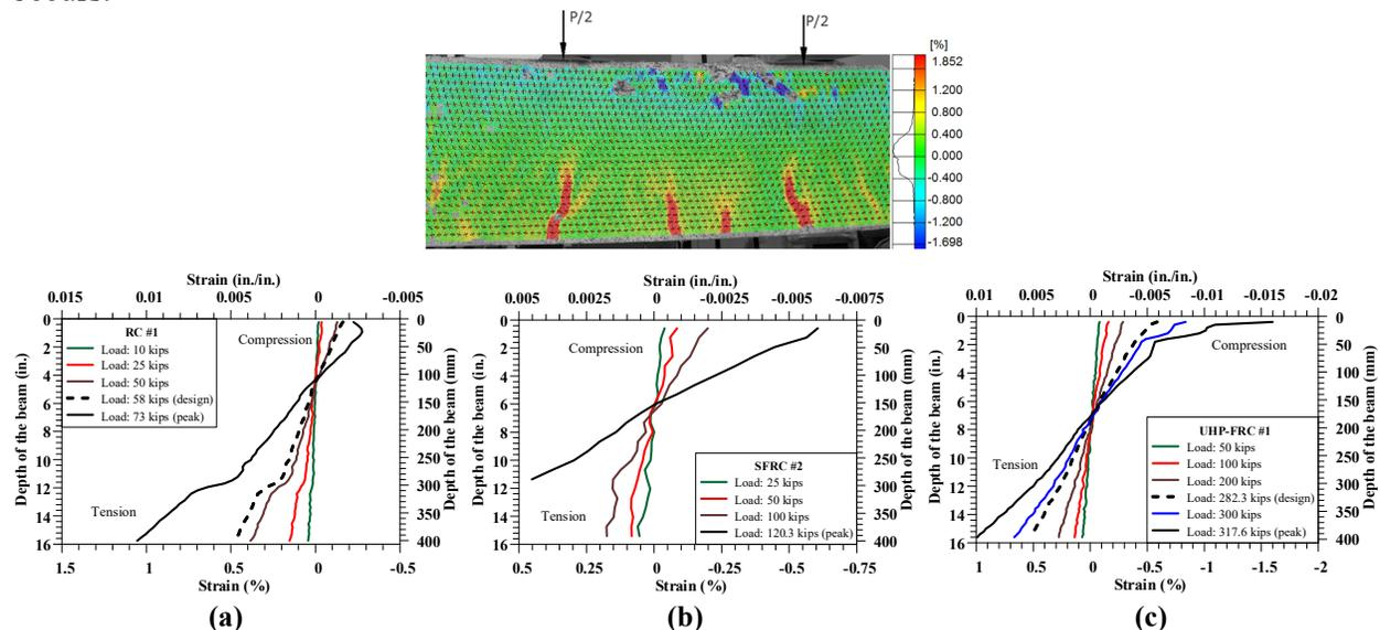
Figure 4: Average measured strains at various loads for the test beams by digit image correlation (DIC) measurement: (a) plain concrete, (b) conventional FRC (0.75%  $V_f$ ), and (c) UHPC (3%  $V_f$ )
