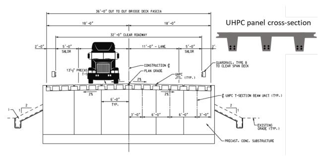
Figure 4: Cross-section of novel UHPC deck bridge
