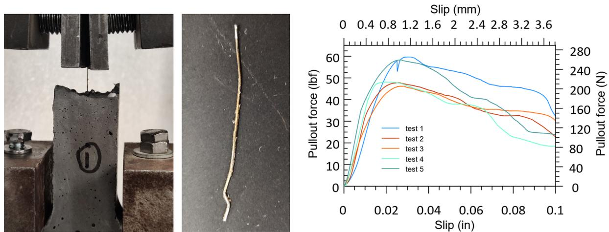
Figure 3: Single-fiber pullout test setup and results
