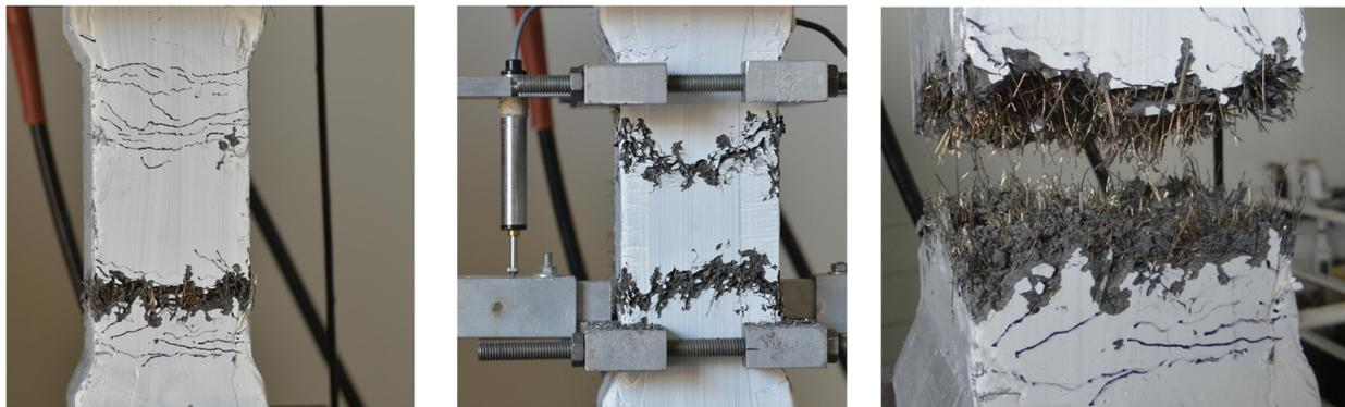
Figure 8: Typical UHP-SIFCON specimens with fiber volume fractions of 7.5%
