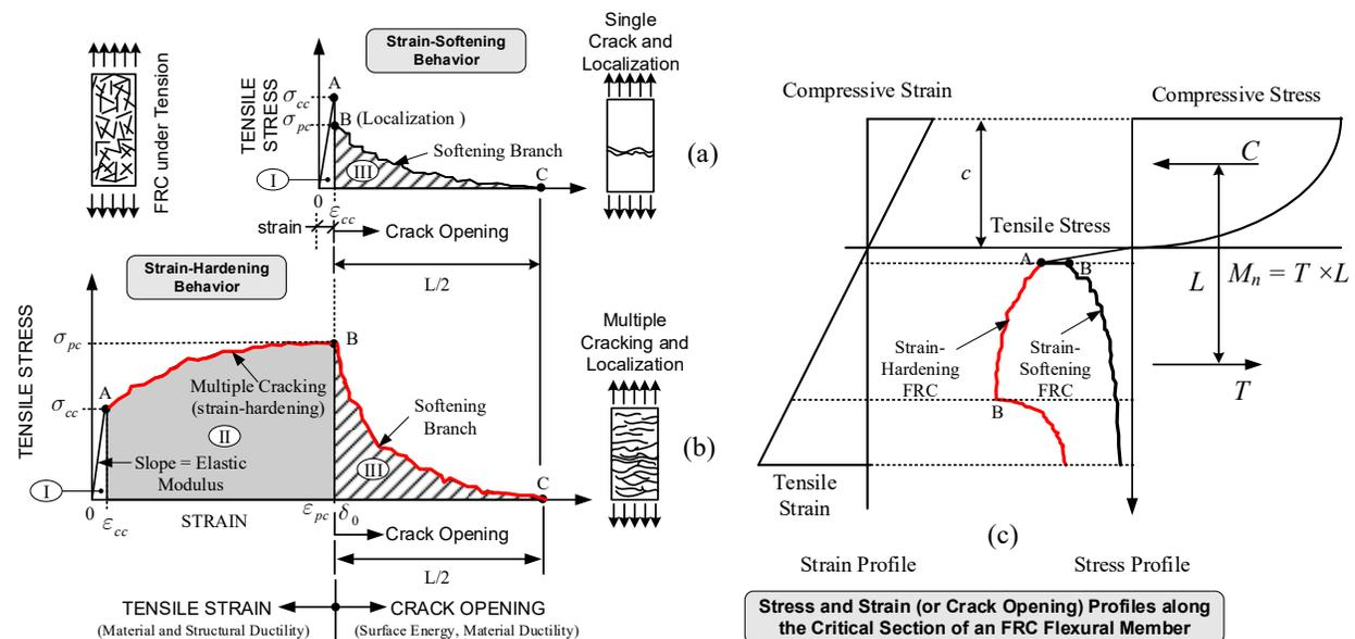
Figure 1: (a) typical tensile stress-strain (crack opening) curve for strain-softening FRCs, (b) typical tensile stress-strain (crack opening) curve for strain-hardening FRCs, (c) bending moment determined by utilizing the tensile stress profile
