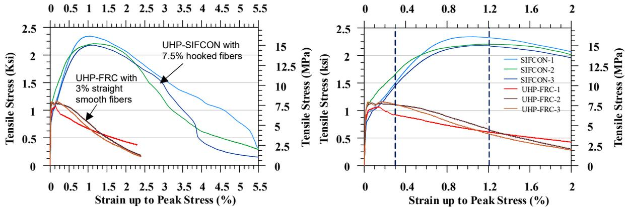
Figure 7: Direct tensile test results of UHP-FRCs with 3% straight smooth fibers and UHP-SIFCONs with 7.5% hooked fibers
