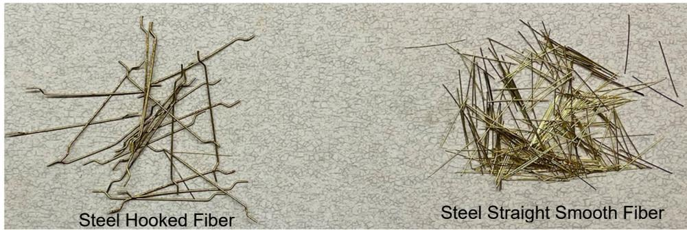
Figure 2: High-strength steel hooked fiber and steel straight smooth fibers used in this study
