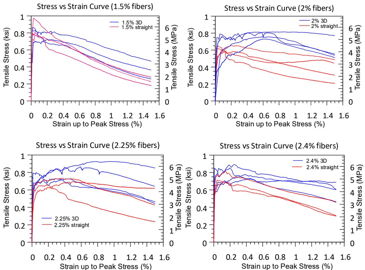
Figure 4: Direct tensile test results of UHP-FRCs with fiber volume fractions of 1.5%, 2%, 2.25%, and 2.4%
