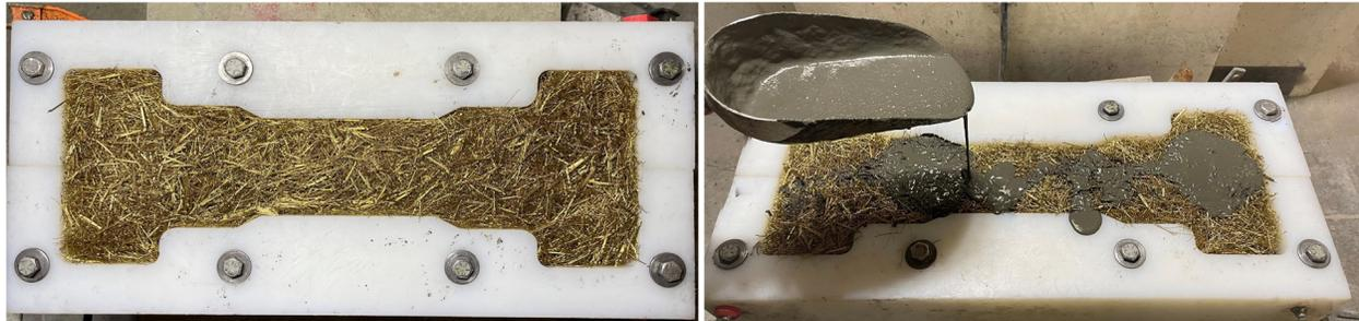
Figure 6: Fabrication of UHP-SIFCON tensile specimen with a fiber volume fraction of 7.5%
