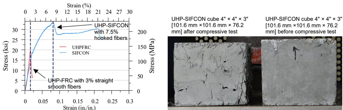
Figure 9: Typical UHP-SIFCON specimens with fiber volume fractions of 7.5%
