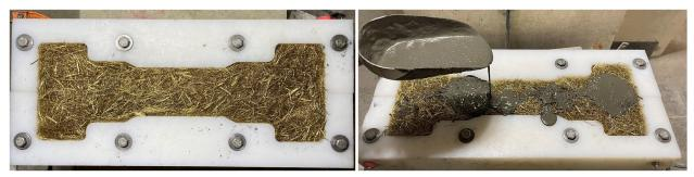
Figure 6: Fabrication of UHP-SIFCON tensile specimen with a fiber volume fraction of 7.5%
