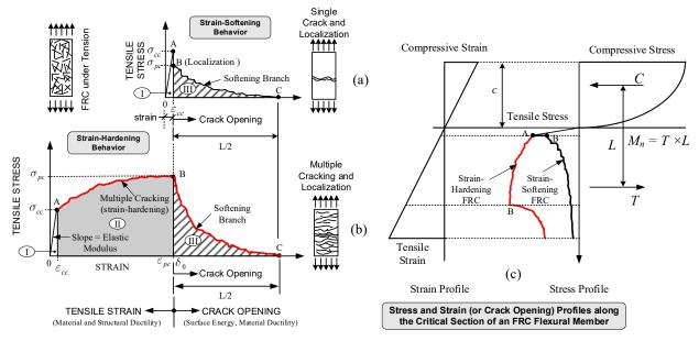
Figure 1: (a) typical tensile stress-strain (crack opening) curve for strain-softening FRCs, (b) typical tensile stress-strain (crack opening) curve for strain-hardening FRCs, (c) bending moment determined by utilizing the tensile stress profile
