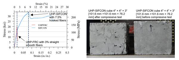
Figure 9: Typical UHP-SIFCON specimens with fiber volume fractions of 7.5%
