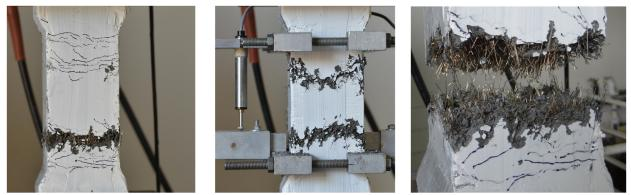
Figure 8: Typical UHP-SIFCON specimens with fiber volume fractions of 7.5%
