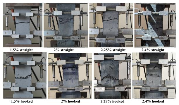
Figure 5: Cracking patterns of UHP-FRCs with fiber volume fractions of 1.5%, 2%, 2.25%, and 2.4%
