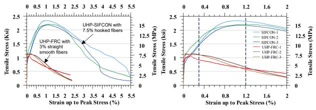
Figure 7: Direct tensile test results of UHP-FRCs with 3% straight smooth fibers and UHP-SIFCONs with 7.5% hooked fibers
