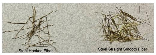
Figure 2: High-strength steel hooked fiber and steel straight smooth fibers used in this study
