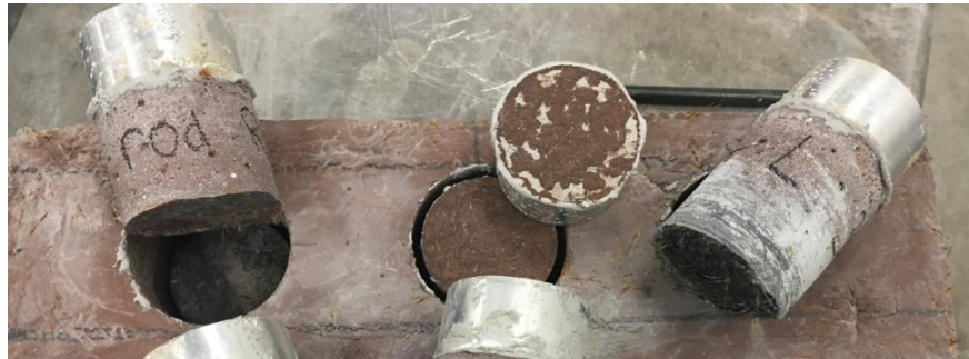
Figure 3. Concrete cores after testing
