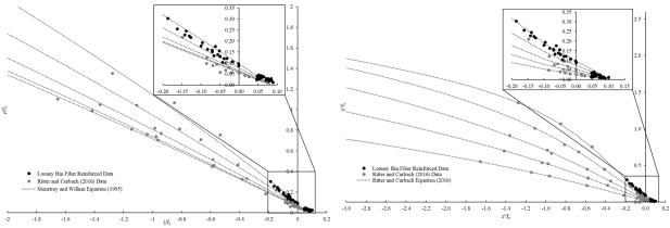
Figure 2 - Menétry and Willam fit (left) and Ritter and Curbach fit (right)
