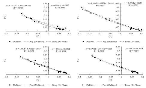
Figure 1 – All collected normalized data for 0% (upper left), 1% (upper right), 2% (lower left), and 4% fiber dosages (lower right)
