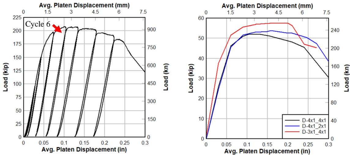
Figure 6. a) Load displacement curve for specimen D-4x1\_4x1, and b) backbone curves for all three specimens.
