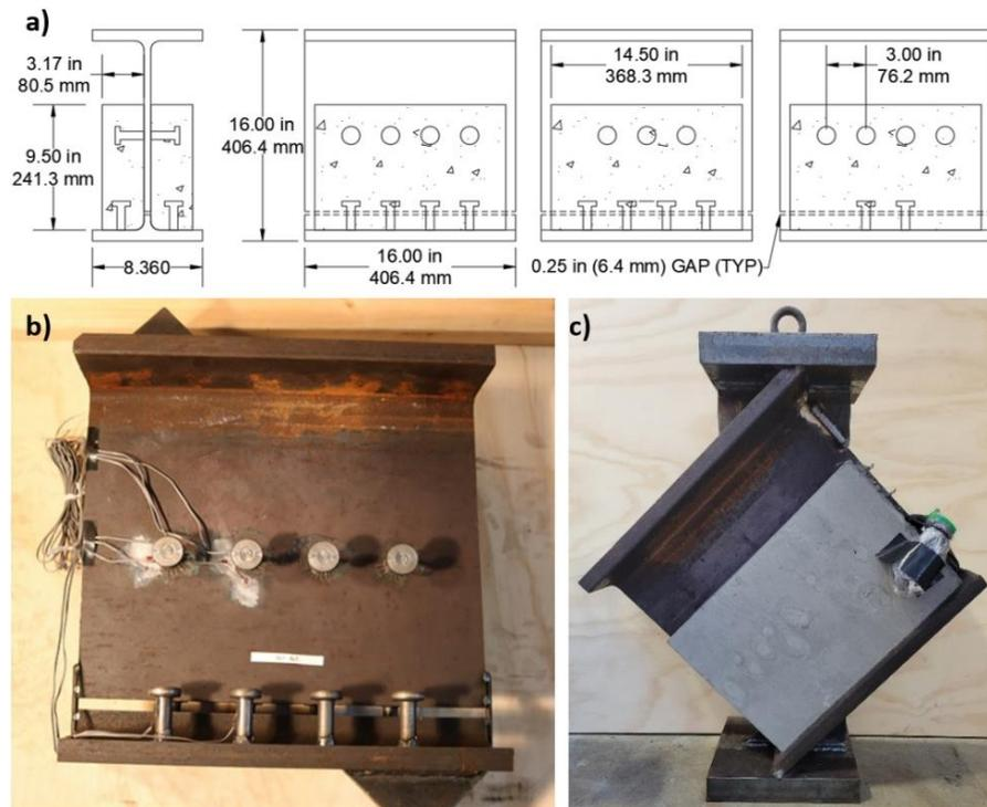
Figure 3. a) CAD model of the three specimen configurations investigated, b) fabricated specimen with strain gauges prior to casting, and c) completed specimen with UHPC panel and support plates.
