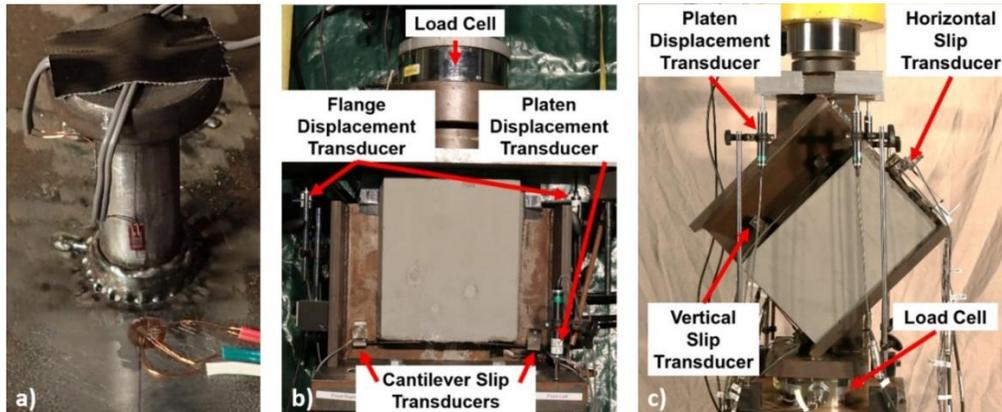
**Figure 4.** a) Typical strain gauging for one stud, b) external sensors and final setup for a push-off specimen, and c) external sensors and final setup for a tilted specimen.
