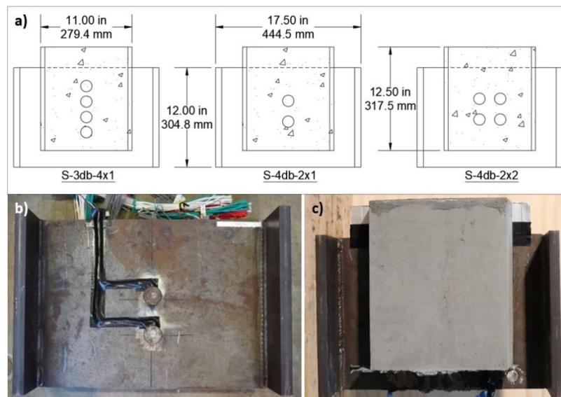
Figure 2. a) CAD model of the three specimen configurations investigated, b) fabricated specimen with strain gauges prior to casting, and c) completed specimen with UHPC panel.
