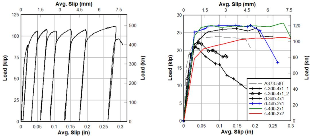
Figure 5. a) Load slip graph from specimen s-4db-2x1, and b) overall backbone curves for all specimens.
