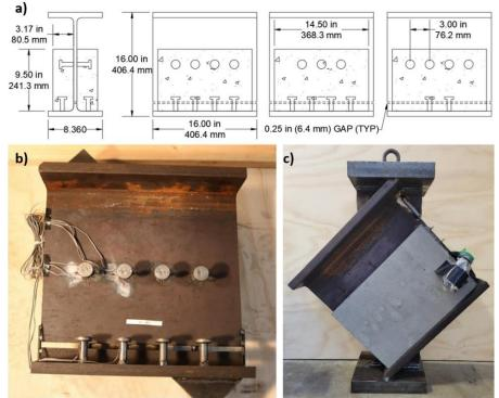
Figure 3. a) CAD model of the three specimen configurations investigated, b) fabricated specimen with strain gauges prior to casting, and c) completed specimen with UHPC panel and support plates.
