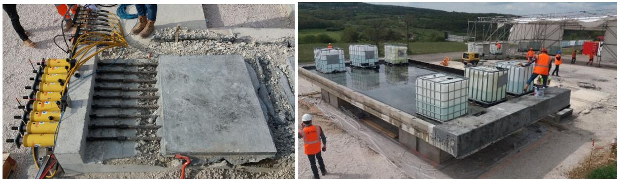
Figure 3: Test of rebars anchoring in UHPC Figure 4: Mockup ponding for waterproofing efficiency testing
