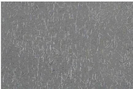
**Figure 7a: UHPC made of preblended constituents. Thixotropic consistence. Surface after hardening and hydroblasting. Fibers oriented along the finisher direction**
