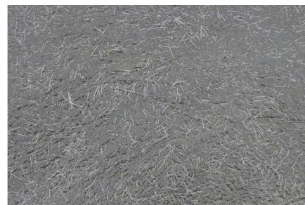
**Figure 7b: UHPC made with same constituents Fluid consistence (+ 2 kg/m<sup>3</sup> SP dosage) Surface aspect. Random fiber orientation**
