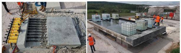
Figure 3: Test of rebars anchoring in UHPC Figure 4: Mockup ponding for waterproofing efficiency testing
