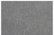
Figure 7a: UHPC made of preblended constituents. Thixotropic consistence. Surface after hardening and hydroblasting. Fibers oriented along the finisher direction
