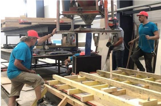
Figure 3: Channel element molding (upside down) and formed on both sides
