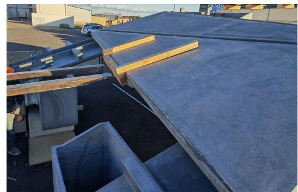
Figure 8: Tests at Innobéton factory: water runoff, shaking of the tiles dropped along the channels
