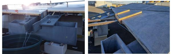
Figure 8: Tests at Innobéton factory: water runoff, shaking of the tiles dropped along the channels
