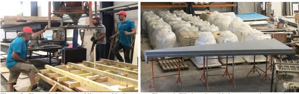
Figure 3: Channel element molding (upside down) and formed on both sides
