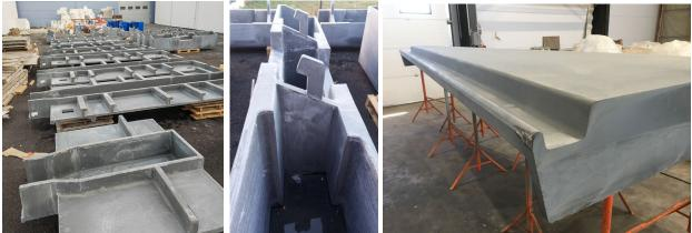
Figure 5: Details of molded elements: channels, boxes with retaining hooks, tiles with side channel
