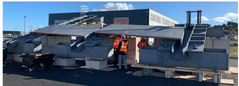
Figure 6: First prototype handling and assembling test at Innobéton factory
