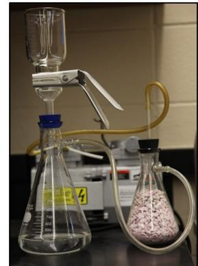
Figure 3. Vacuum filtration test setup.
