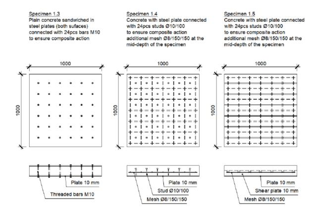
Figure 2. Detailed description of the specimens 1.3 to 1.5 (2.3 to 2.5)
