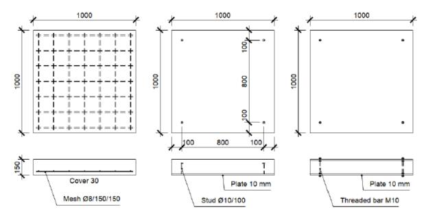
Figure 1. Detailed description of the specimens 1.0 to 1.2 (2.0 to 2.2)
