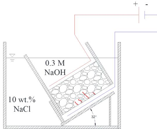
**Figure 2 Modified rapid non-steady chloride migration test**
