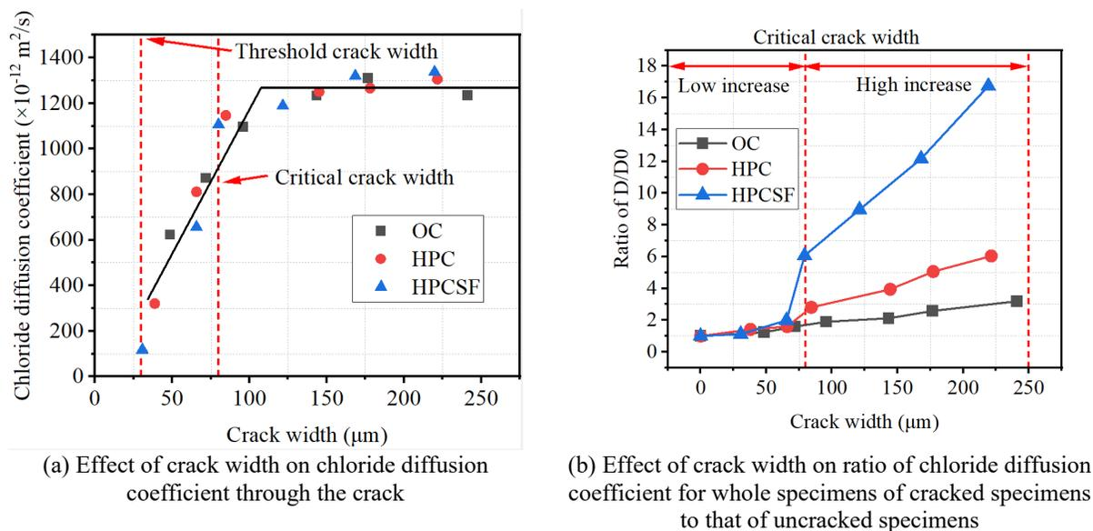
**Figure 1 Crack width against chloride diffusion coefficient for concrete (Djerbi et al.)**
