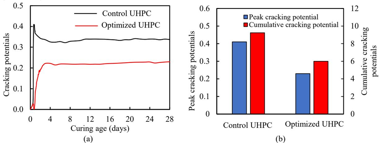
**Figure 1.** Summarized cracking potentials of controlled UHPC and optimized UHPC.
