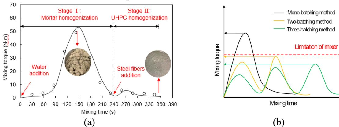
Figure 3. Mixing torque evolution of mixing UHPC: (a) mono-batching method; (b) multi-batching method.
