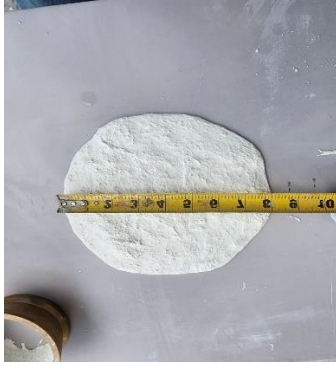
Figure 3. The 8” spread for the right flow
