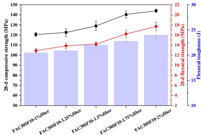
**Figure 3. 28-d compressive and flexural strengths and toughness of optimized UHPC mortars**
