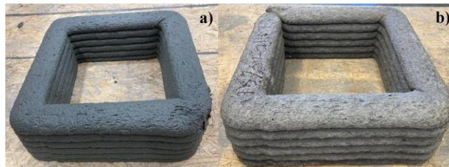
**Figure 4. Printability of optimized UHPC; (a) captured before setting and (b) captured after hardening**
